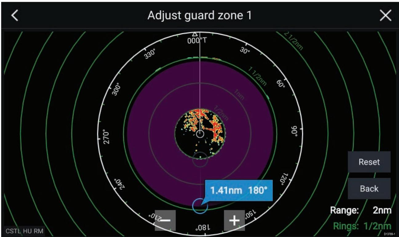
Adjust the guard zone size by dragging the inner and outer perimeter end points (circles) to the desired locations.
