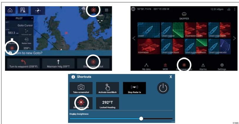
You can disengage your autopilot at any time by selecting the **Disengage pilot icon**.
