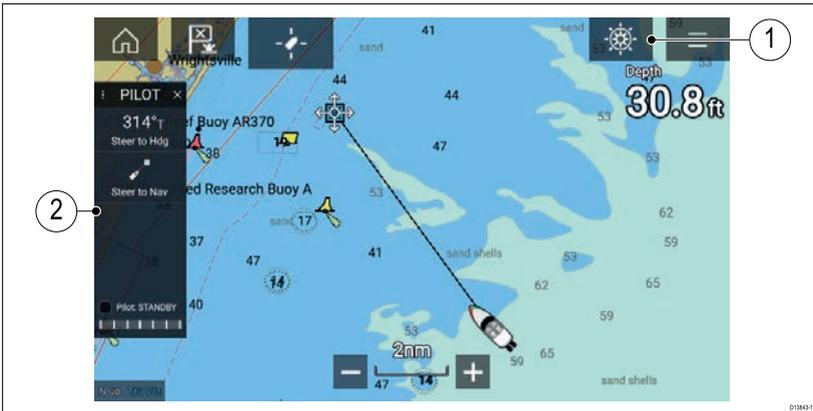
1. **Pilot icon** — With **Autopilot control** enabled, the Pilot icon is displayed onscreen; selecting the icon displays the Pilot sidebar. When the Autopilot is engaged the Pilot icon is replaced with the Disengage pilot icon.
