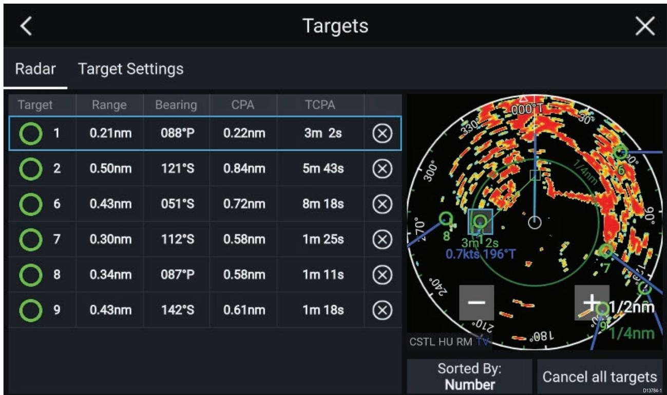
Selecting a target from the list will highlight the selected target in the app pane on the right of the screen.
